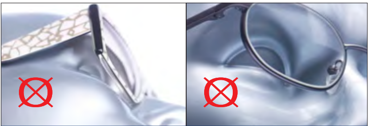
Unsuitable protective glasses: The pictures above show two good examples of incorrectly fitting glasses that allow radiation to directly hit the lens of the eye undeterred.
