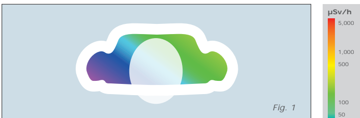
Condition for the examiner with the new protective shield without a curtain: The light blue area indicates a high exposure dose in the upper body area as a result of the radiation that has traveled underneath the radiation protective shield.
